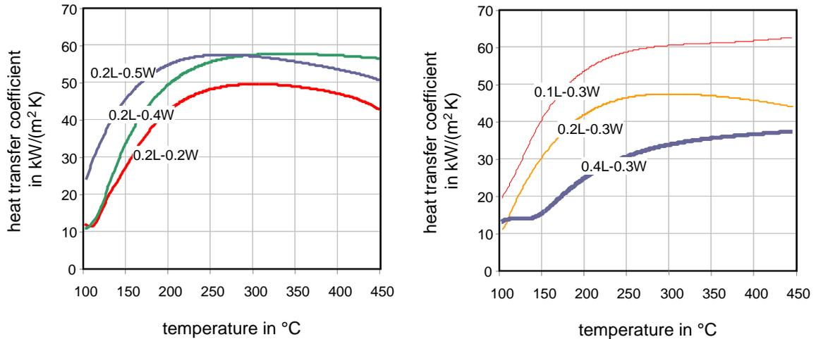
Fig. 2 – Heat transfer coefficients determined for the centre of a spray cooled disc of the alloy AlSi11Mg for various spray types; nozzle type SUJ12, 1/8JJAU (Spraying Systems Co.); left: influence of rising water pressure; right: influence of rising air pressure
